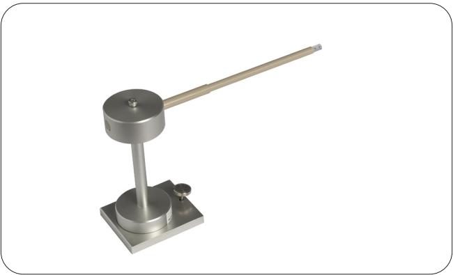
Figure 7. 8 mm FOV specimen holder
