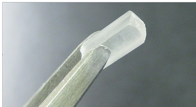
Figure 4. Example of a polymer sample cut to have a flat top and bottom, for measurement by both DSC and FT-IR. This sample began as a "chip" (depending on the resin used, the common name used for unprocessed polymer may vary between "flake, chip, pellet, etc.")
