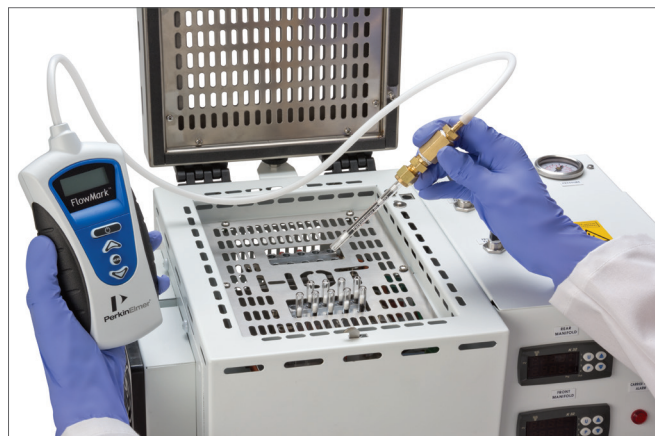
Figure 1. Even if the oven is partially loaded, gas will only flow to the cells that contain TD tubes, leaving you with no wasted purge gas and flexibility in your work flow.
