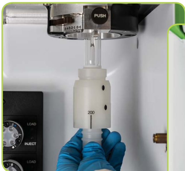
Installing a ZipTorch on Avio 200
