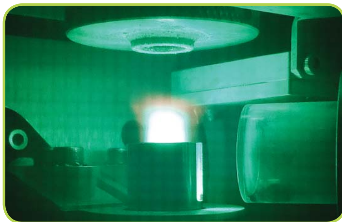
Nitride torch while nebulizing Yttrium on the Avio ICP
